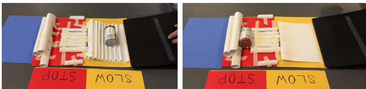
These images show a student’s design for the slow and stop zone during testing with the small “car”. For the design in the left image, the car stopped in the “slow down” zone and thus this design did not meet the specified criteria (not a good design). For the design shown in the right image, the car successfully stopped in the “stop” zone, which meets the criteria and is thus a good design.
