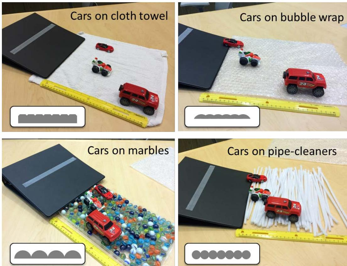
Images of three different sized cars traveling on four different surfaces. The distance traveled in each case is directly affected by the surface. The insets show the approximate cross-section (side-view) of the surfaces, illustrating the different texture (smooth to bumpy) of the different surfaces.
