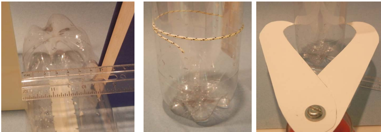
Figure 8. Measuring the diameter of a cylinder (in this case a plastic water bottle): Left photo – place the cylinder flat on a table; place two books (rectangles) upright on the table and move them to touch opposite sides of the cylinder; measure the distance between the edges of the books with a ruler. Center photo – wrap a string around the cylinder to measure the circumference; divide the circumference by \pi (3.1416) to get the diameter. Use a caliper (such as the homemade one in the photo) to measure the width of the cylinder, then use a ruler to determine the distance between the two points on the caliper.
